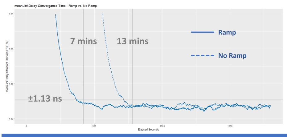
Without Ramping, meanLinkDelay takes 13 mins to settle, vs 7 mins with Ramping
