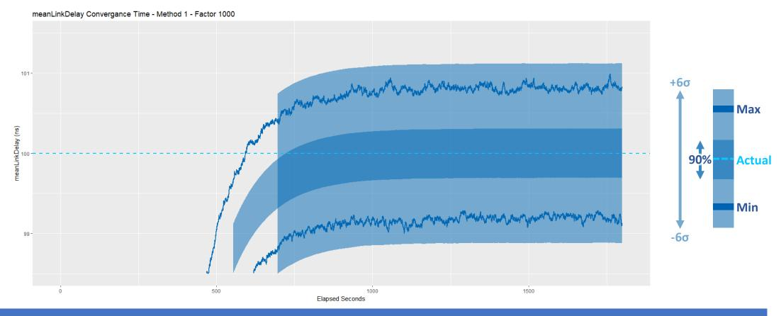
Without correct initialisation (and without ramping) meanLinkDelay error can take 10 mins to stabalise
