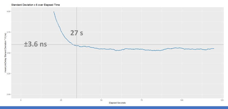
Factor of 100 settles to ±3.6 ns after 27 s (verses ±3.39 ns for factor of 1000; ±1.13 ns after 7 mins)
