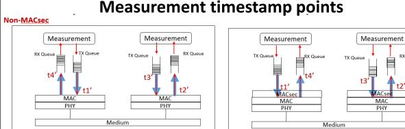
PFC Headroom = (t2'+ PFC reaction delay + r\_tx\_shim layer delay ) – (t1'-PFC invocation delay-PFC frame - l\_tx\_shim layer delay ) +t4'-t3' + 2\*(Max Frame)
