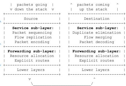
DetNet functionality is implemented in two adjacent sub-layers in the protocol stack
