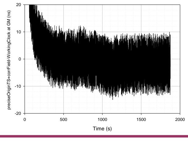
Case 4, Replication 1 rateRatio field of transmitted Sync message by DUT minus actual rate ratio of DUT working clock relative to Working Clock at GM at transmission of Sync message Detail of initial transient not shown on scale of plot Node 3
