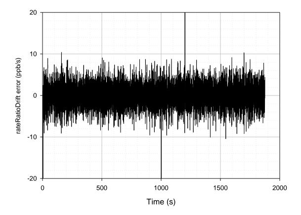
Case 3, Replication 1 Filtered dTE (PTP End Instance), Node 3 Full detail of initial transient not shown on scale of plot
