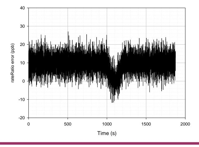
Case 4, Replication 1 rateRatioDrift field of transmitted Sync message by DUT minus actual rate ratio drift rate of DUT working clock relative to Working Clock at GM at transmission of Sync message Detail of initial transient not shown on scale of plot Node 3
