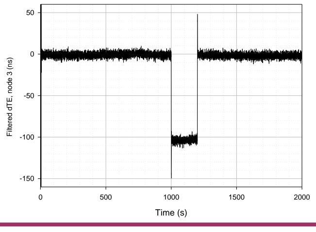
Case 2, Replication 1 Filtered dTE (PTP End Instance), Node 3 Detail of initial transient, period of clock drift, and transients when clock drift starts and stops not shown on scale of plot
