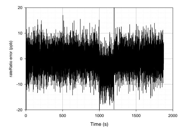
Case 2, Replication 1 rateRatioDrift field of transmitted Sync message by DUT minus actual rate ratio drift rate of DUT working clock relative to Working Clock at GM at transmission of Sync message Detail of initial transient not shown on scale of plot Node 3
