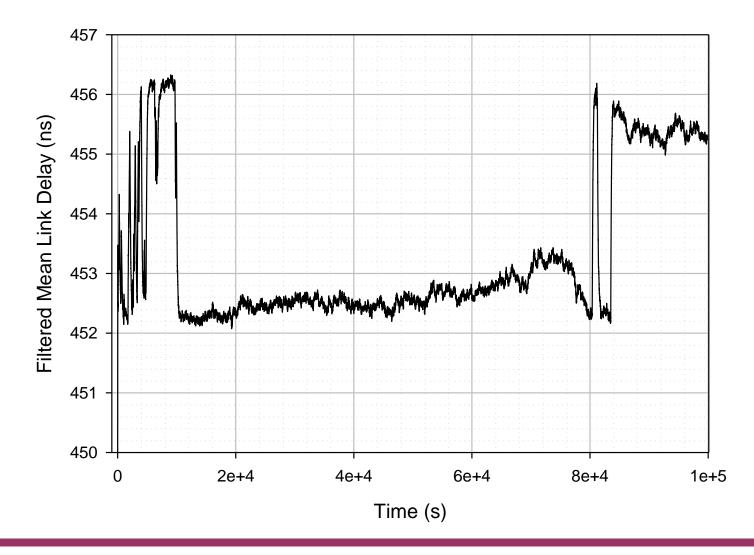
Case01b - Mean Link Delay before IIR Filtering - Replication 1
