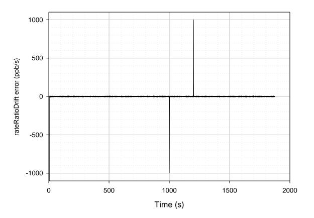
Case 3, Replication 1 rateRatioDrift field of transmitted Sync message by DUT minus actual rate ratio drift rate of DUT working clock relative to Working Clock at GM at transmission of Sync message Detail of initial transient and transients when clock drift starts and stops not shown on scale of plot Node 3
