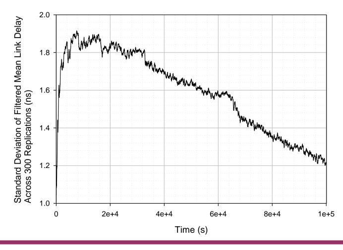
Case01c Standard deviation of mean link delay before IIR filtering, across 300 replications (Ensemble average)
