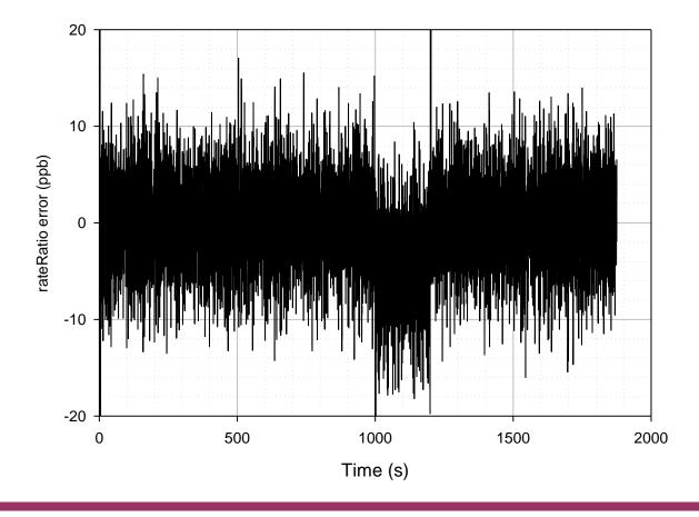
Case 3, Replication 1 rateRatioDrift field of transmitted Sync message by DUT minus actual rate ratio drift rate of DUT working clock relative to Working Clock at GM at transmission of Sync message Detail of initial transient not shown on scale of plot Node 3
