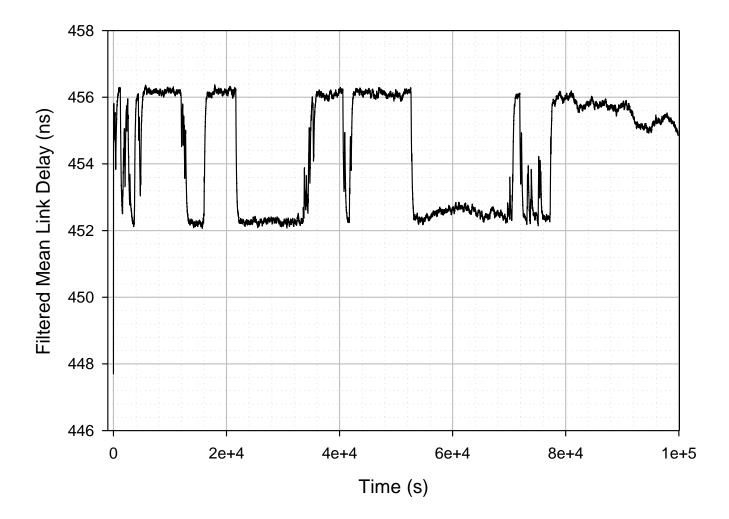
Case01 - Mean Link Delay before IIR Filtering - Replication 1
