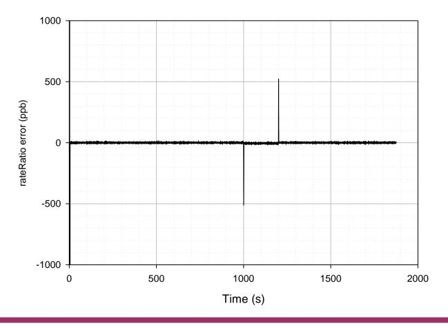
Case 2, Replication 1 rateRatio field of transmitted Sync message by DUT minus actual rate ratio of DUT working clock relative to Working Clock at GM at transmission of Sync message Detail of initial transient and transients when clock drift starts and stops not shown on scale of plot Node 3
