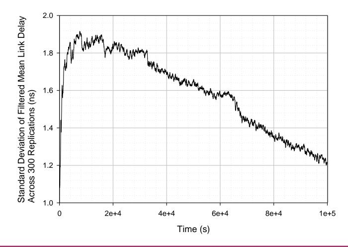
Case01 Standard deviation of mean link delay before IIR filtering, across 300 replications (Ensemble average)
