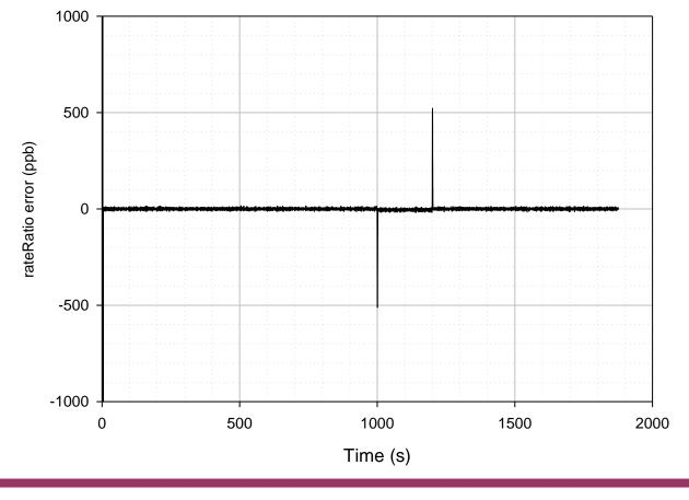
Case 3, Replication 1 rateRatio field of transmitted Sync message by DUT minus actual rate ratio of DUT working clock relative to Working Clock at GM at transmission of Sync message Detail of initial transient and transients when clock drift starts and stops not shown on scale of plot Node 3
