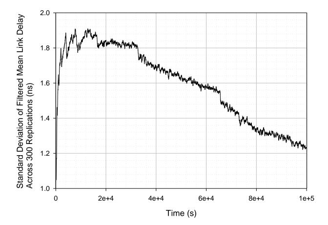
Case01b Standard deviation of mean link delay before IIR filtering, across 300 replications (Ensemble average)
