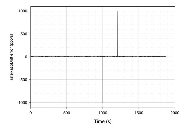
Case 2, Replication 1 rateRatioDrift field of transmitted Sync message by DUT minus actual rate ratio drift rate of DUT working clock relative to Working Clock at GM at transmission of Sync message Detail of initial transient and transients when clock drift starts and stops not shown on scale of plot Node 3
