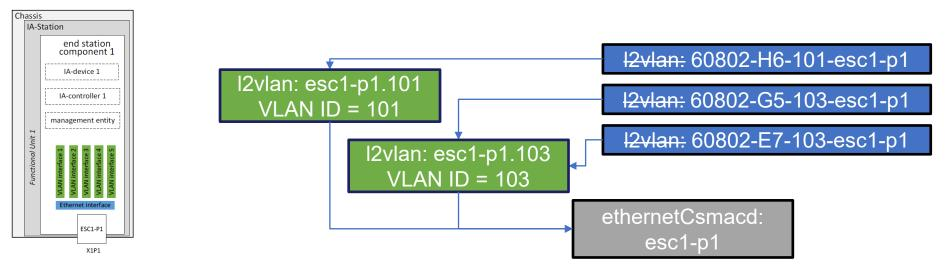
Figure 7 – IETF Interfaces used for Traffic Type Translation
