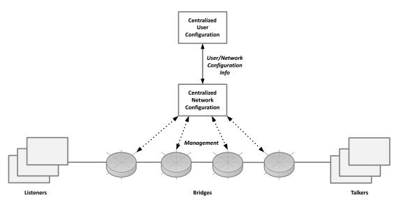
Figure 46-3—Fully centralized model
