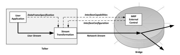
Figure 46-4—Example of Stream transformation in Talker end station
