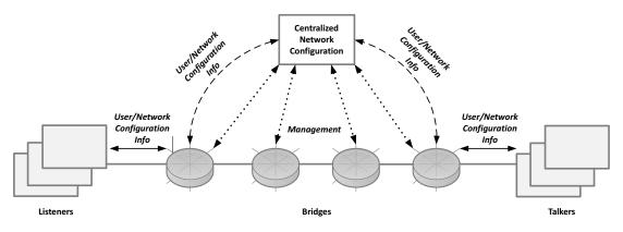
20 Figure 46-2 provides a graphical representation of the centralized network/distributed user model.
