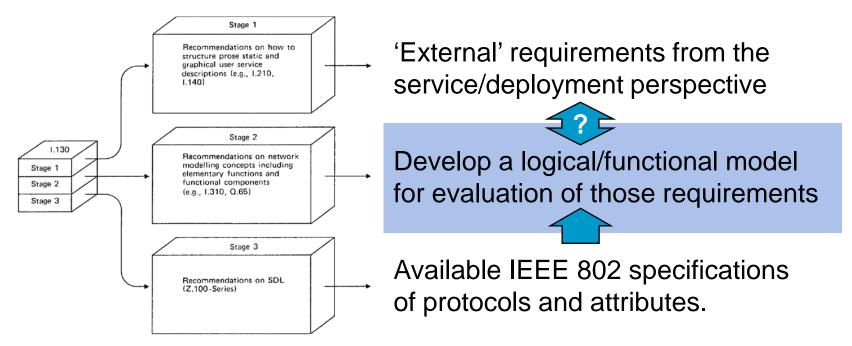
A 'Stage 2' specification provides a mapping of the existing IEEE 802 protocols to a functional network model, which facilitates easier evaluation and better understanding of end-to-end behavior.
