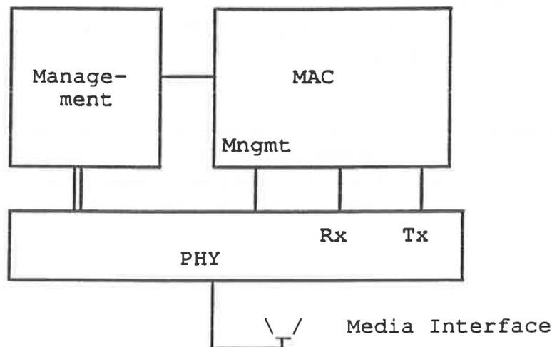
The objective is to develop one MAC for a range of different PHY's. Although the MAC may contain PHY specific provisions, it is intended to provide for a generic functional MAC/PHY interface.
