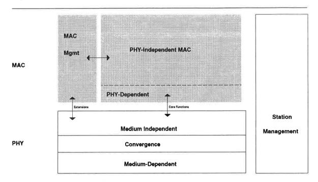
The interface between the MAC and PHY is depicted above as a set of core functions with PHY-specific extensions. This of course can be implemented in a variety of different ways. It is probably best to define the extensions for the various PHYs in a uniform fashion, allowing a common interface to be used for all PHYs (though each PHY would only implement its specific extension functions). The MAC/PHY interface could then easily be optionally exposed.
