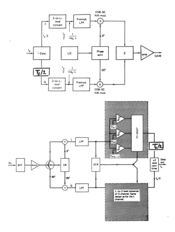
Fig. 1. Flexible bit rate/QUAD modulator/demodulator nonlinearly amplified (NLA) or linear offset OQPSK, constant envelope FQPSK and QAM systems for bit rates in the 1 Mb/s to 3 Mb/s range with BER =  $10^{-5}$  for  $E_b/N_o$  less than 16 dB [References: 1-13; 21].
