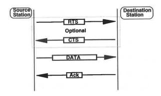
RTS and CTS include "duration" of subsequent data/ack exchange
