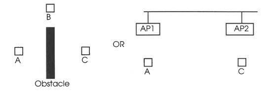
The Current Proposal does not refer to how does station A know how to reach station C
