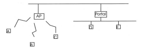
The 802.11 stations (A, B, and C) will be connected to Ethernet Stations (D, and E), through the AP and a Portal.
