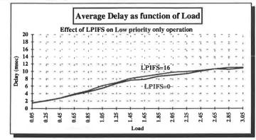
No difference at low Loads, minor impact during higher loads, showing lower Throughput.
