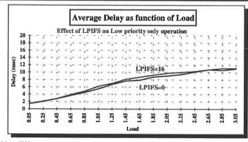
No difference at low Loads, minor impact during higher loads, showing lower Throughput.
