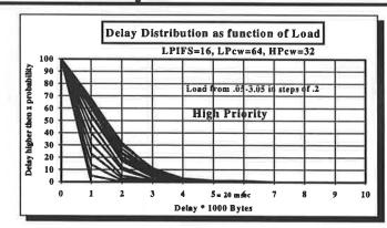
• 20 msec max delay can be met even in high priority overload case.
