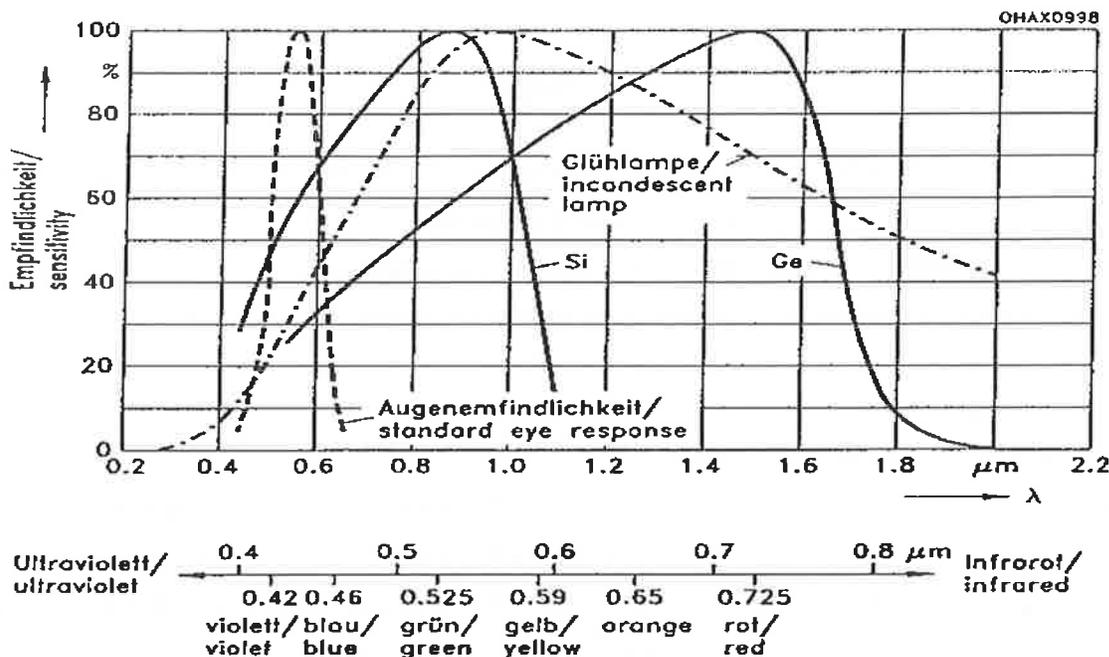
Fig. 2: Relative sensitivity of different light-sensitive detectors
