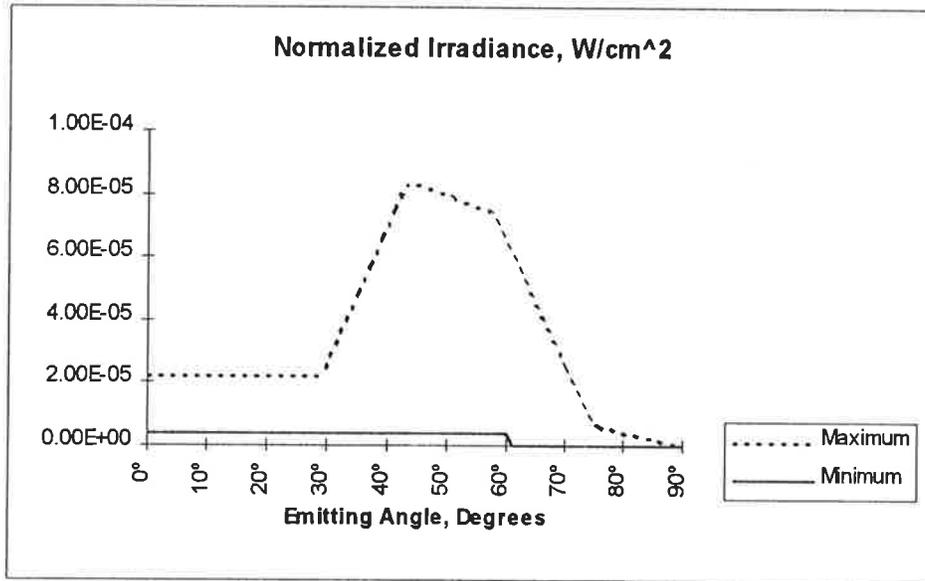
Figure 12-4: Emitter radiation pattern mask.
