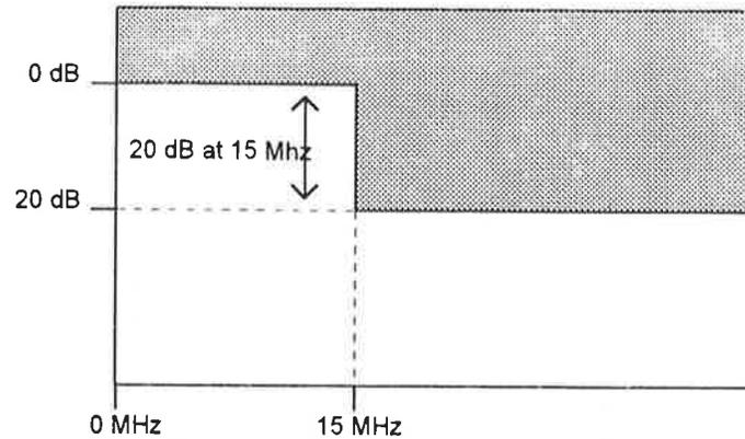
Figure 12-5: Transmit spectrum mask.
