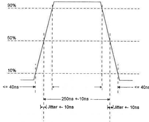
Figure 12-3: Basic Pulse Shape
