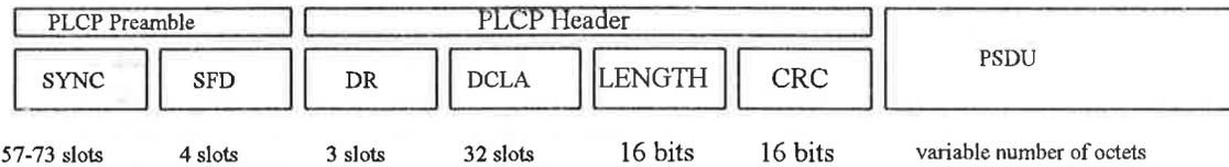
**Figure 12-1: PDU PLCP Frame Format**
