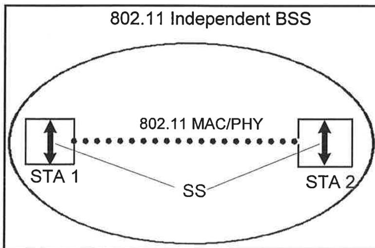
Figure 2-10: Logical Architecture of an Independent BSS
