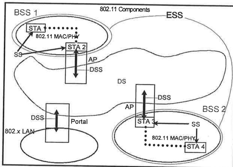
**Figure 2-7: Complete 802.11 Architecture**
