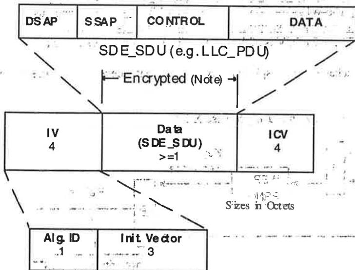
Note: The encryption process has expanded the SDE\_PDU by 8 Octets, 4 for the Initialization Vector (IV) field and 4 for the Integrity Check Value (ICV). The ICV is calculated on the Data field only.
