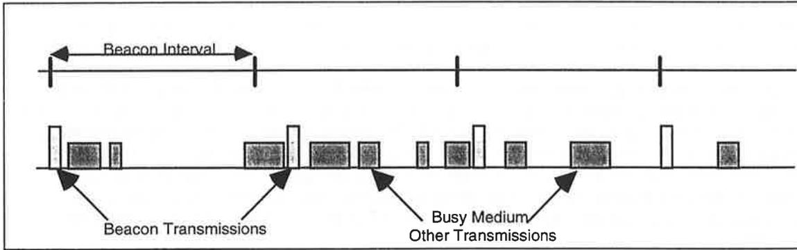
Figure 8-1 — Beacon transmission on a busy network.
