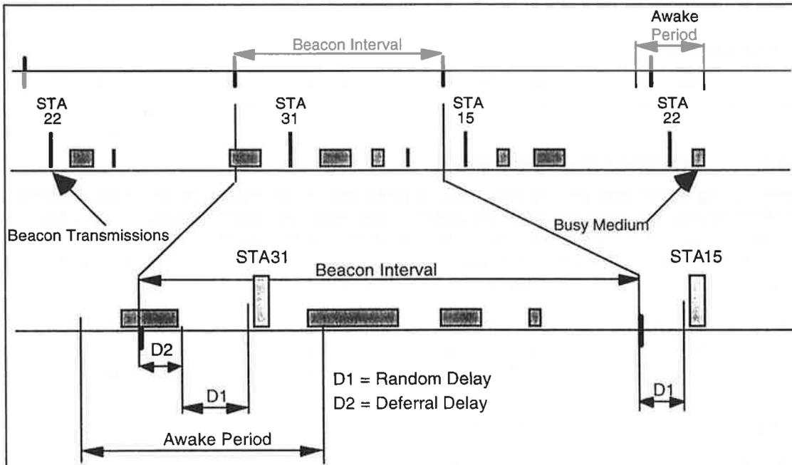
Figure 8-2 — Beacon transmission in an Ad Hoc network.
