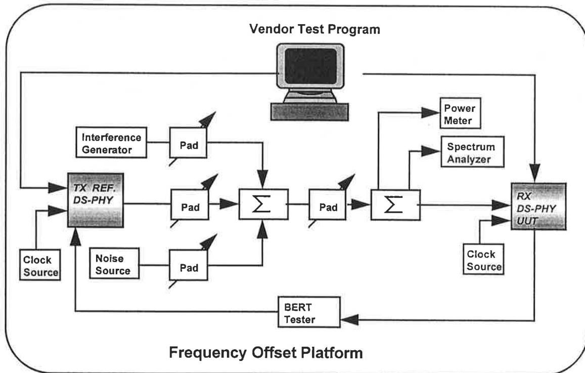
Figure 3. RF Test Bed For Offset Measurements.
