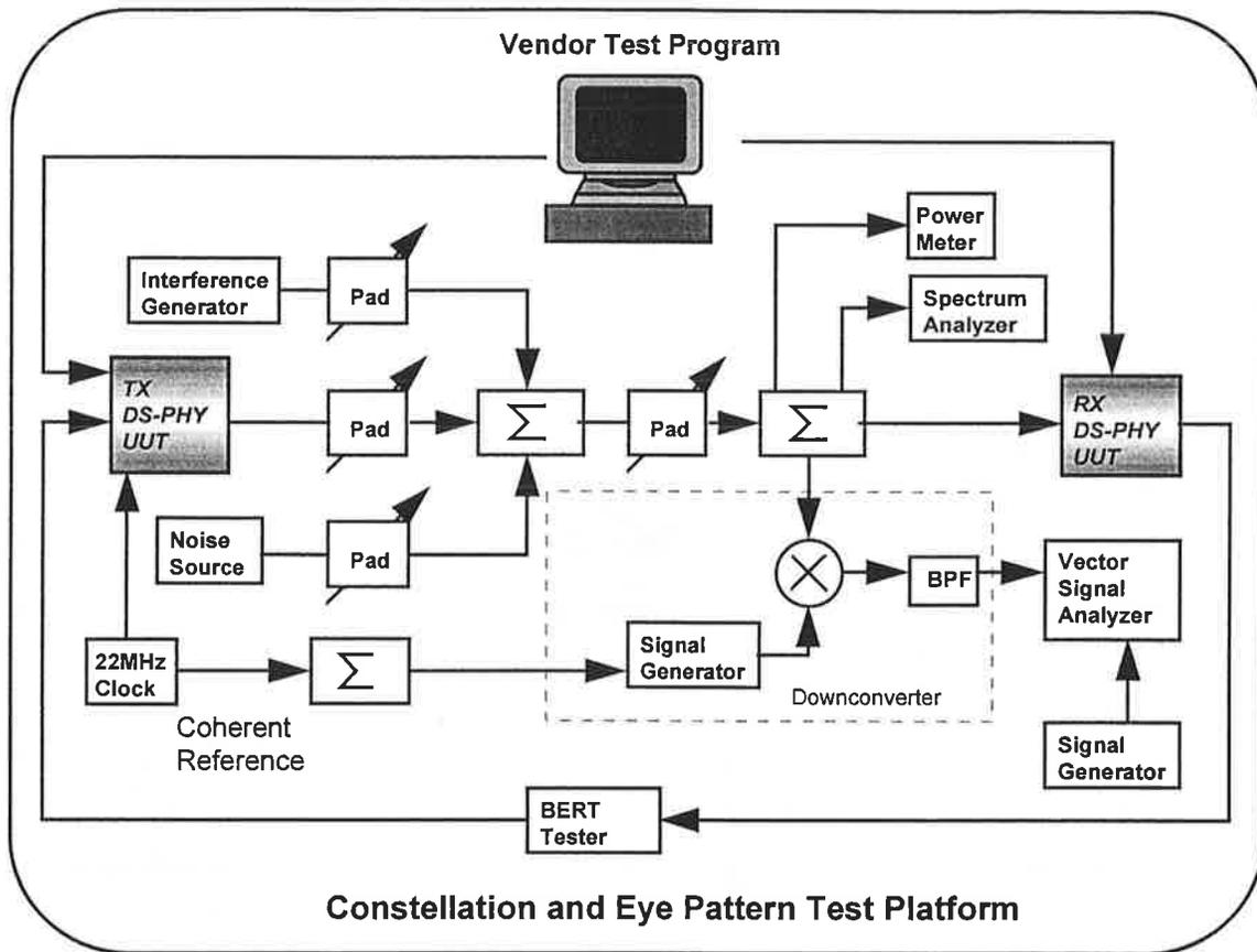
**Figure 4. Constellation and Eye Pattern Conformance Test Bed**
