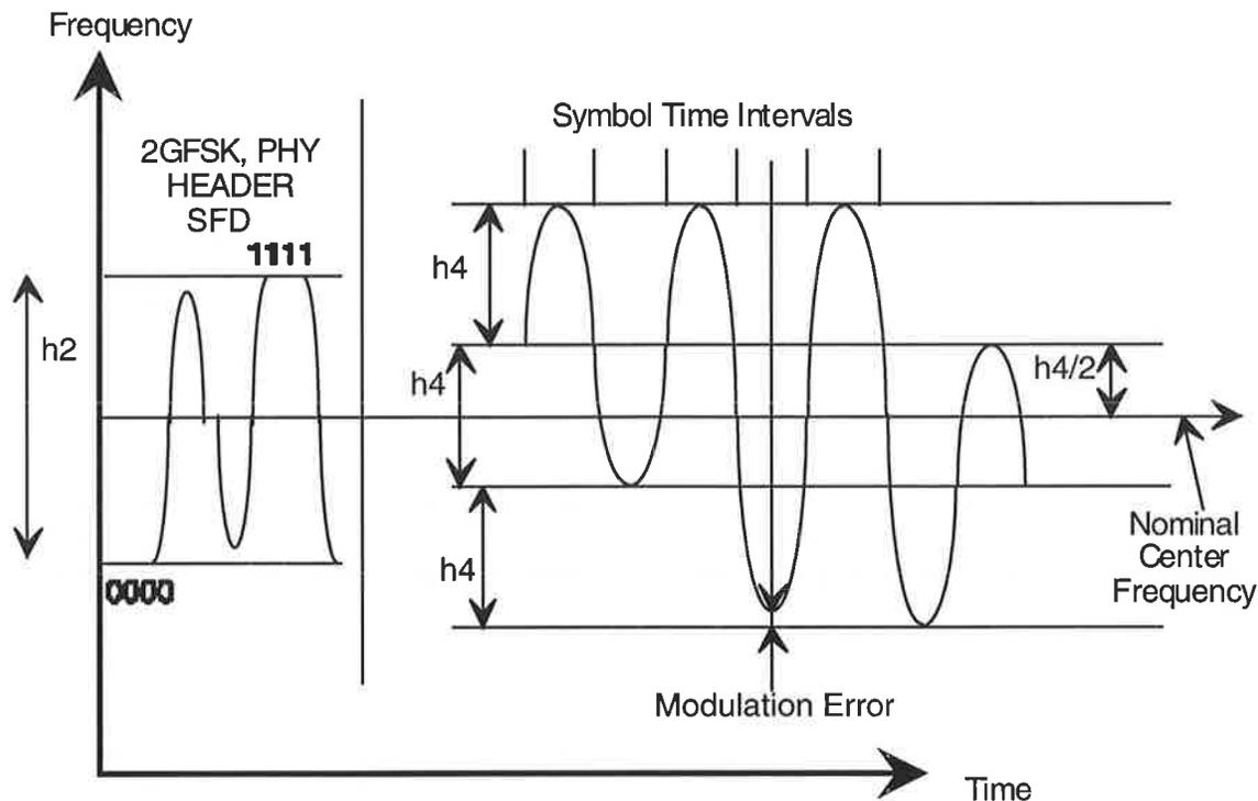
Figure C, 4 Level GFSK Transmit Modulation
