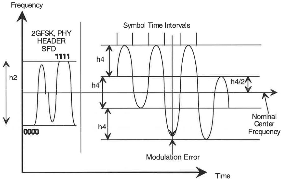
Figure C, 4 Level GFSK Transmit Modulation
