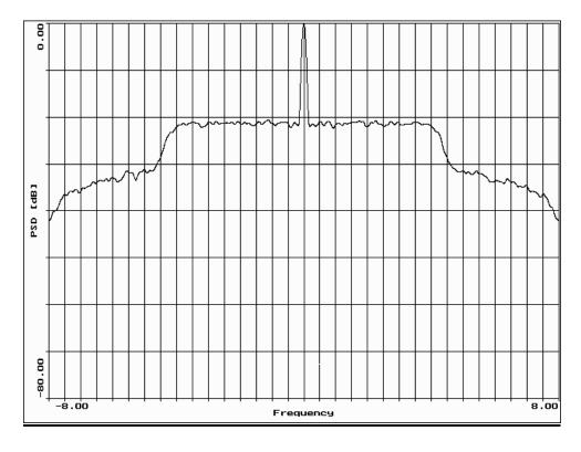
Figure 2: PSD of the proposed signal, simulated with 100 KHz RBW
