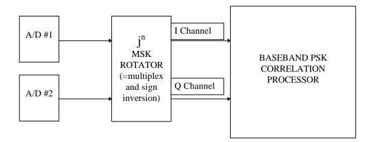
With this technique, an existing correlation processor for PSK signals can be made to process MSK waveforms with no other changes than the "rotator" shown.
