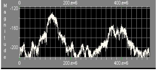
The transmit amplifier operating point was approximately 1.7 dB into gain compression.
