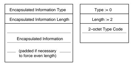
Figure 1. Encapsulated Information Element Format and Values for Type 2 Ethernet
