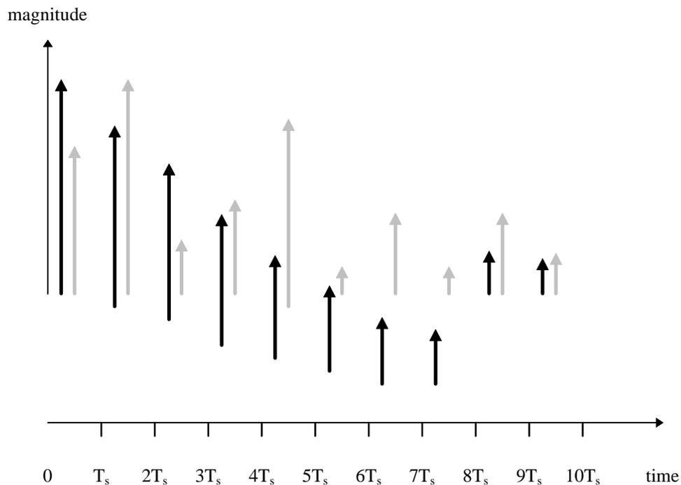
Fig 1: Channel impulse response; black illustrates average magnitudes, gray illustrates magnitudes of a specific random realization of the channel; the time positions of black and gray samples are staggered for clarity only.
