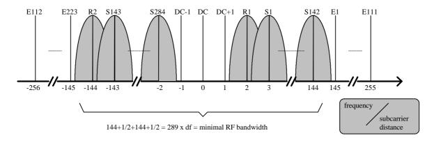
Figure 3: OFDM subcarrier allocation (frequency spectrum) in the equivalent lowpass domain.
