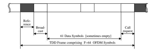
Figure 5: TDD-frame structure with one reference symbol per frame for synchronisation purposes.
