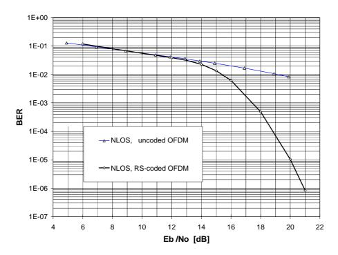
Figure 11: Uncoded and coded bit error rates of the overall Median physical layer for a Non Line of Sigth (NLOS) multipath channel (target environment for future system). HPA nonlinearities, LO phase noise, synchronisation are included.
