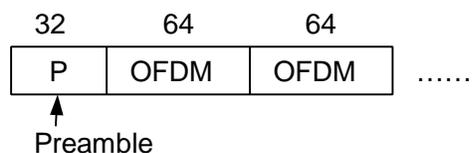
Fig.1 Preamble Structure
