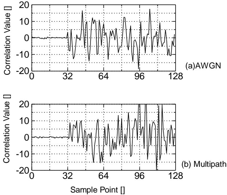
Fig.2 Waveform of [PN preamble + OFDM Data Symbol] (Only real part)
