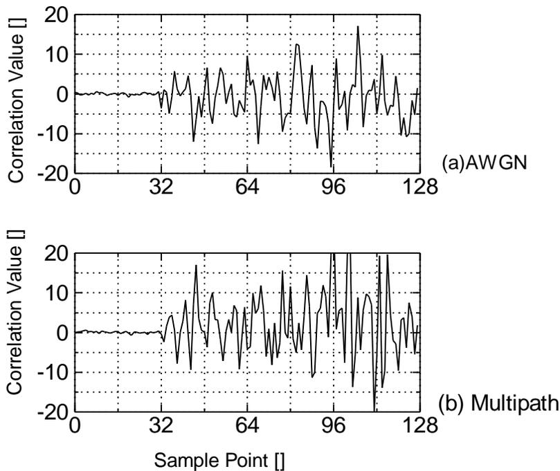
Fig.3 Waveform of [OFDM preamble + OFDM Data Symbol] (Only real part)
