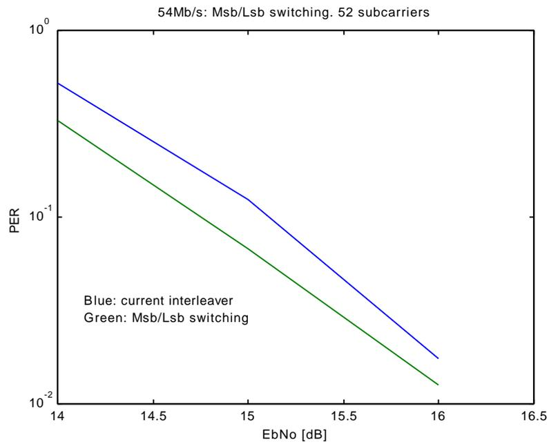
Figure 6 - 54 Mb/s modulation
