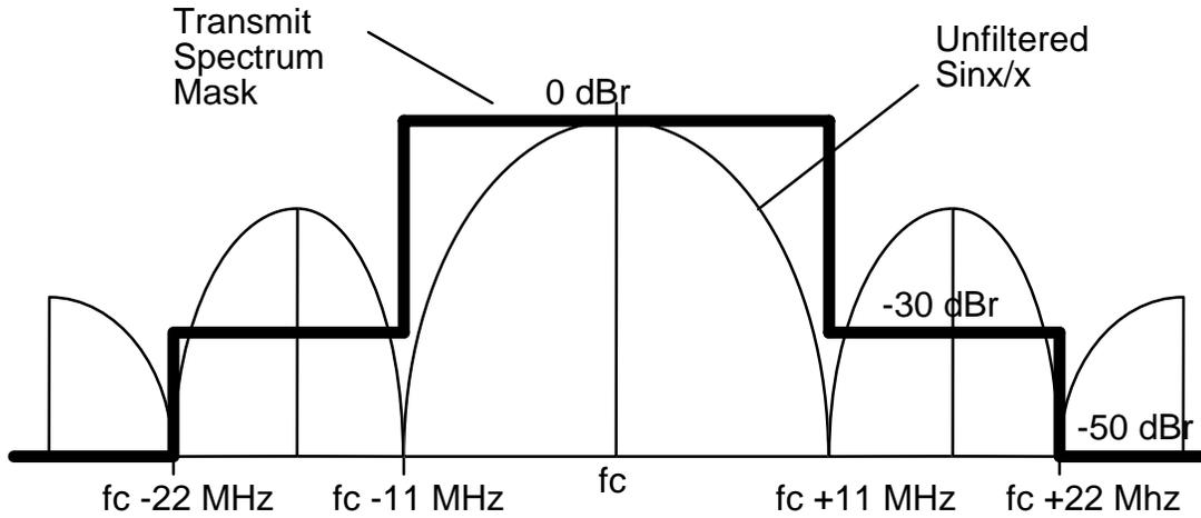
Figure 15—Transmit spectrum mask
