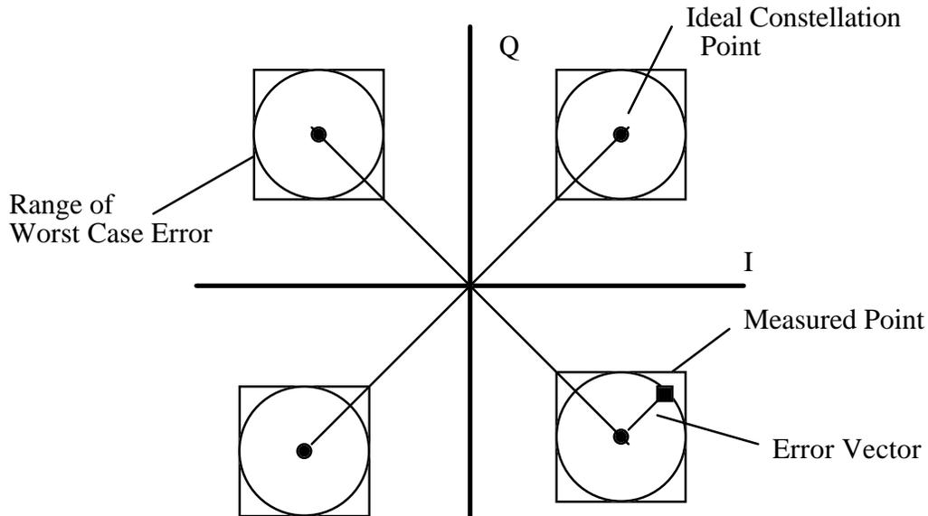
Figure 18—Modulation Accuracy Measurement Example
