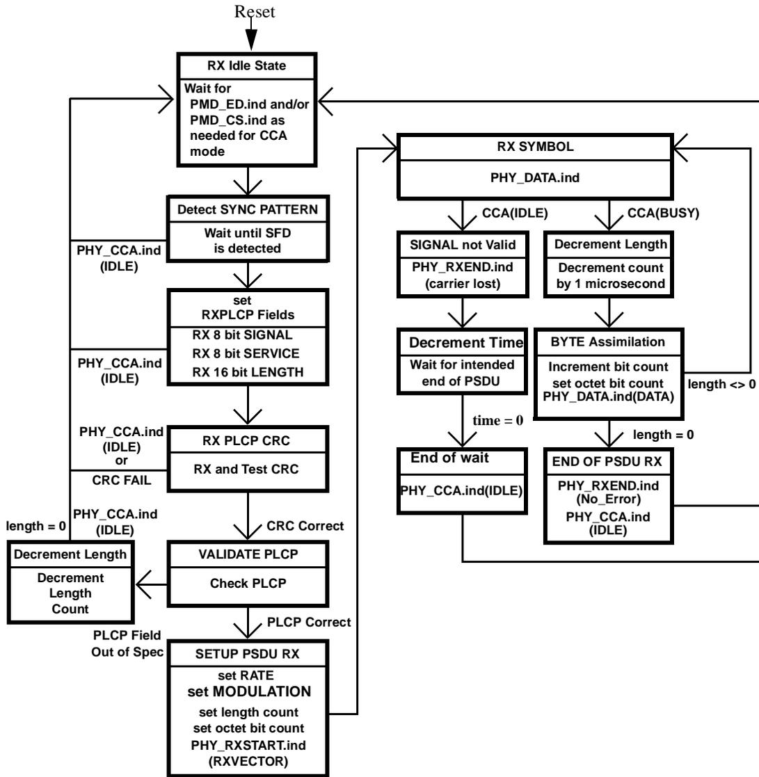
Figure 10—PLCP receive state machine
