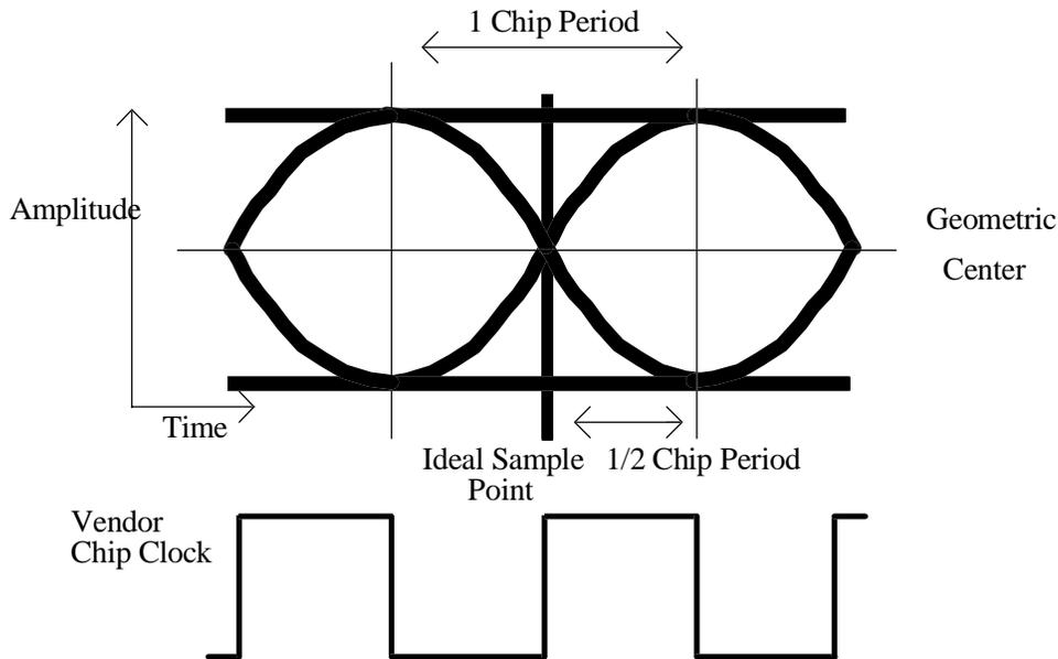
Figure 19—Chip Clock Alignment with Baseband Eye Pattern
