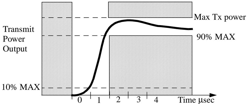
Figure 16—Transmit Power-On Ramp
