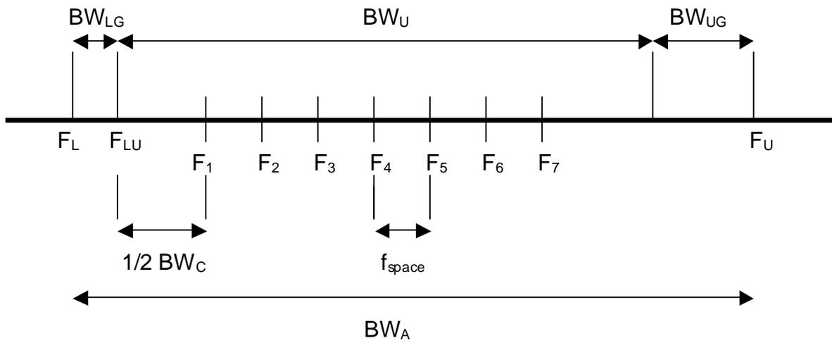
Figure 1, Parameters for Channel Allocation
