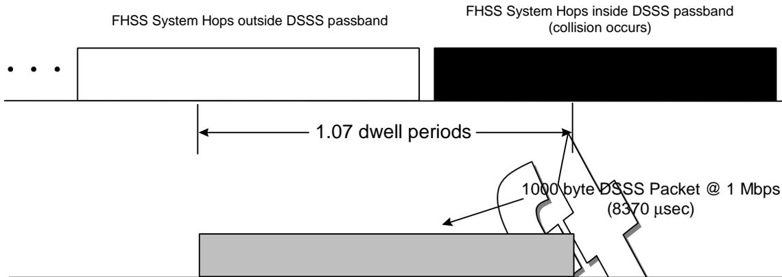
**Figure 3.0-1 Probability of Collision Depends on Hop Rate**
