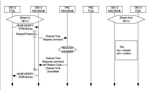
Figure 118 - MSC for a denied stream modification
