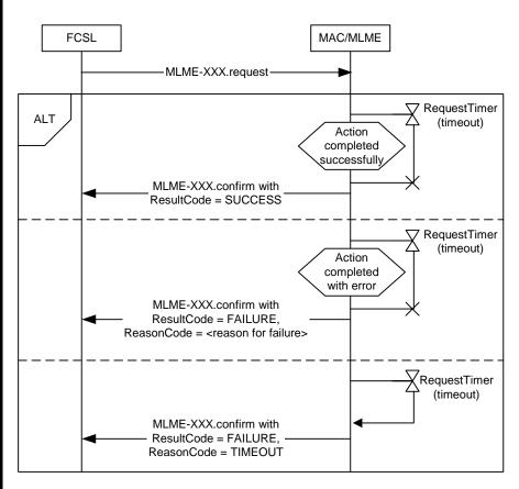
Figure 91 - MSC showing the possible results of a primitive request
