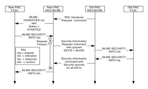
Figure 149—Message sequence chart for New PNC-Old PNC Security Information transfer
