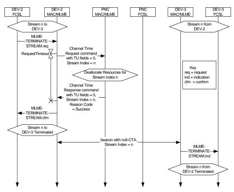
Figure 120 - MSC of source DEV-2 requesting termination of its stream
