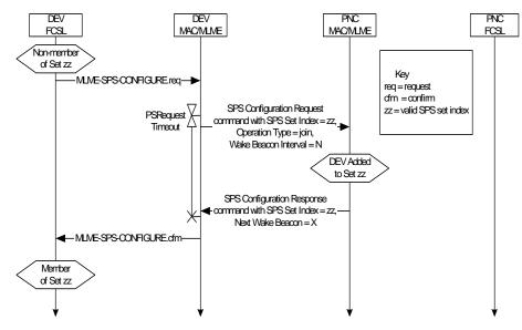
Figure 142 - MSC showing a DEV joining an existing SPS set
