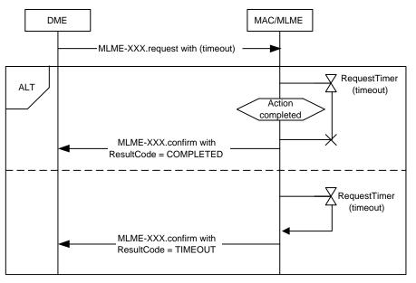
Figure 91 - MSC showing examples of primitive timers
