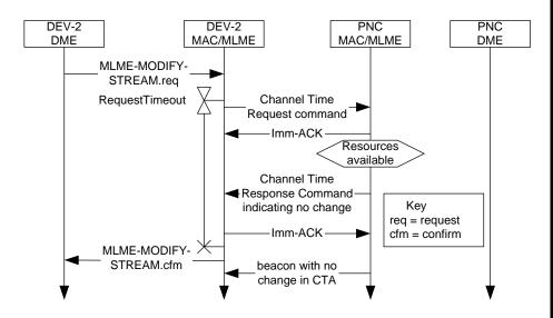
Figure 118 - MSC for a denied stream modification
