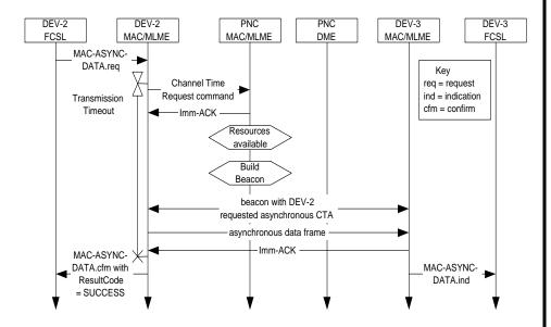
Figure 123 - MSC for reserving asynchronous data channel time
