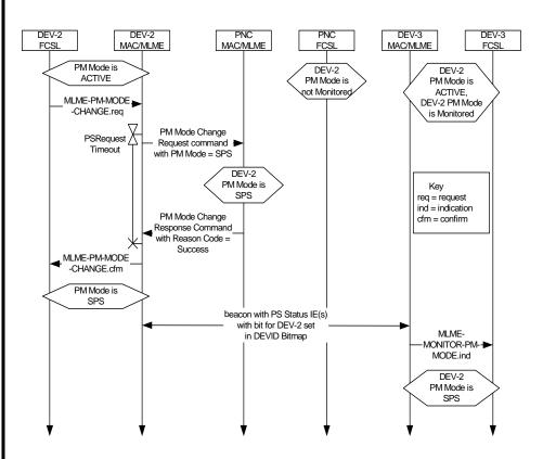
Figure 144 - MSC showing DME initiated PM mode change from ACTIVE to an SPS mode
