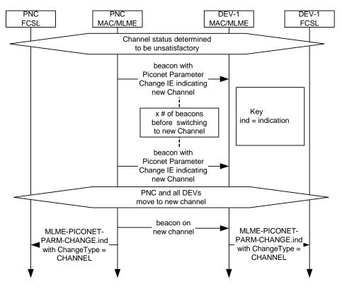
Figure 135 - MSC for changing the channel for a piconet
