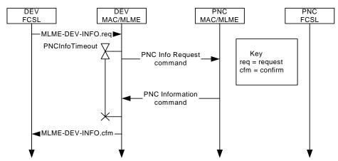
Figure 127 - MSC for acquiring information regarding a specific DEV or all of the DEVs from the PNC using the PNC Information Request and PNC Information commands
