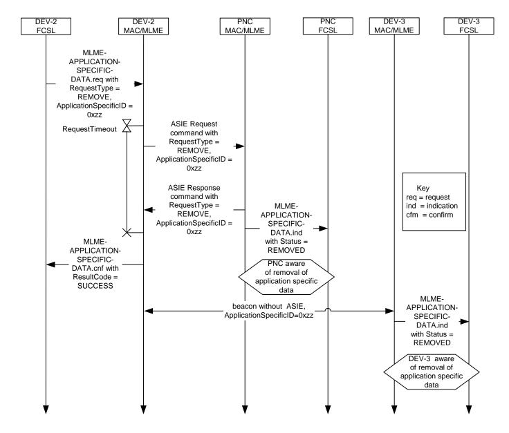
New - DEV removing application specific data from a beacon
