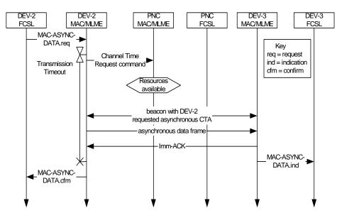
Figure 123 - MSC for reserving asynchronous data channel time
