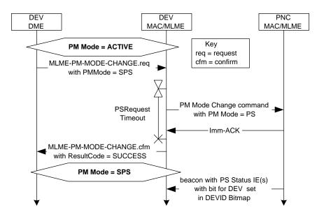
Figure 144 - MSC showing DME initiated PM mode change from ACTIVE to an SPS mode
