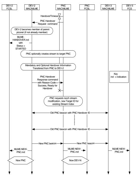
Figure 95 - Successful PNC handover in a dependent piconet
