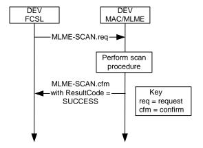
Figure 92 -MSC for scan operation
