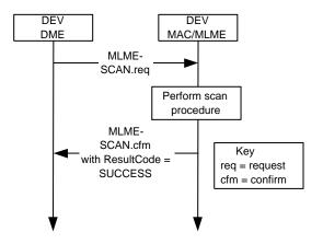
**Figure 92 -MSC for scan operation**
