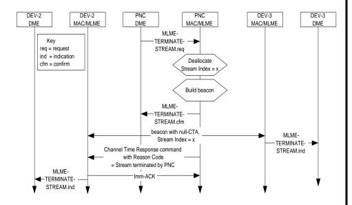
Figure 122 - MSC of PNC terminating a stream
