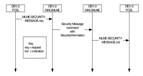
Figure 150—Message sequence chart for sending security information with the Security Message command
