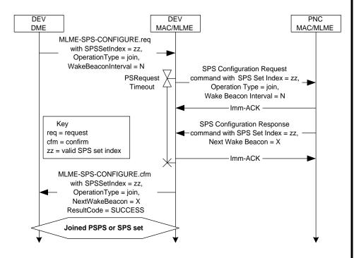
Figure 142 - MSC showing a DEV joining an existing SPS set
