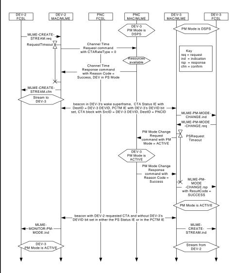
Figure 147 - Message sequence showing MLME initiated PM mode change from DSPS to ACTIVE in response to a new chanel time allocation
