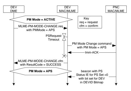
Figure 145 - MSC showing DME initiated PM mode change from ACTIVE to APS
