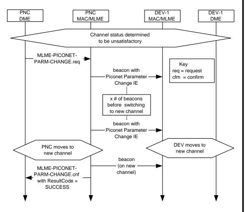
Figure 135 - MSC for changing piconet parameters
