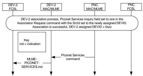
Figure 103 - PNC sending the Piconet Services command to a newly associated DEV in response to a request in the association process
