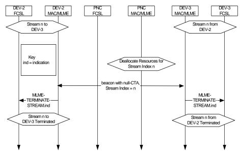
Figure 122 - MSC of PNC terminating a stream
