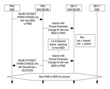
Figure 134 - MSC for changing either the PNID or BSID for a piconet
