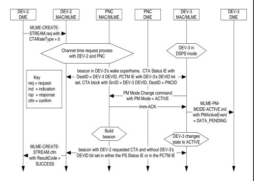
Figure 147 - Message sequence showing MLME initiated PM mode change from DSPS to ACTIVE in response to a new changl time allocation
