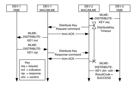
Figure 152—Message sequence chart for peer-to-peer key distribution
