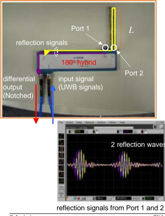
By setting the electric length  $L (=c\delta = c/f_n; m=2)$ , a notch at arbitrary frequency  $f_n$  is obtainable, in principle.
