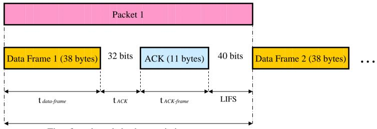
Time for acknowledged transmission,  $t_{packet}$
