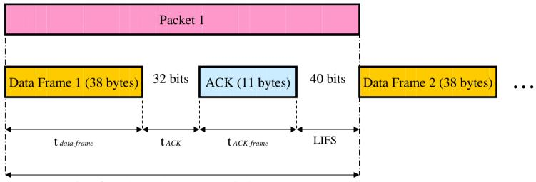
Time for acknowledged transmission,  $t_{packet}$
