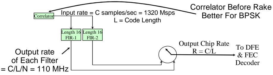
NEW PROPOSAL CHANGES TO Complexity = (16 multipliers) \* (N=2 branches) \* (400 gates per 3-bit mult) \* (<u>110 MHz</u>) 85.5MHz = 26k Gates (including adders and overhead)
