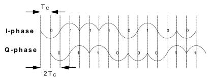
Figure 26—Sample baseband chip sequences with pulse shaping
