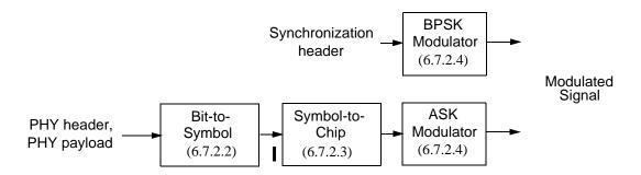
Figure 22—Modulation and spreading functions
