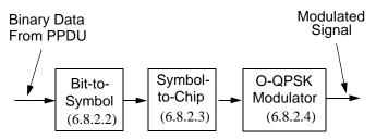
Figure 24—Modulation and spreading functions
