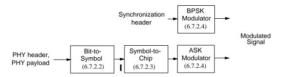
Figure 22—Modulation and spreading functions
