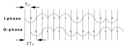
Figure 26—Sample baseband chip sequences with pulse shaping
