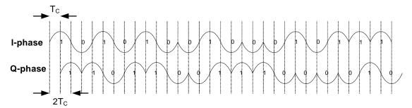
Figure 20—Sample baseband chip sequences with pulse shaping
