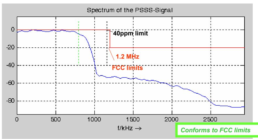
Simulations of the relative PSD in dB for the PSSS 250-1600 signal: With precoding, at 1,600 kchip/s, 250 kbit/s, +/- 40ppm, 50% PA drive, as specified in draft TG4b PHY text
