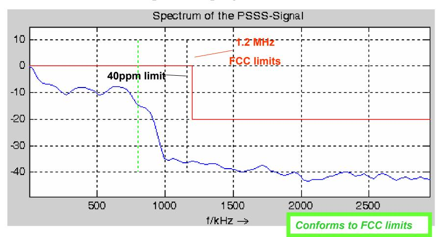
Simulations of the relative PSD in dB for the PSSS signal: With precoding, at 1,600 kchip/s, 250 kbit/s, +/- 40ppm, 100% PA drive, as specified in draft TG4b PHY text
