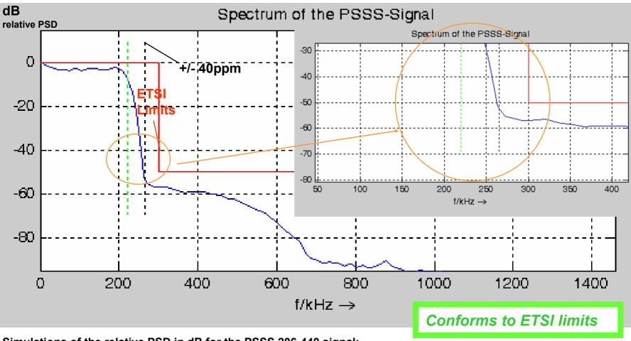
Simulations of the relative PSD in dB for the PSSS 206-440 signal: With precoding, at 440 kchip/s, 206 kbit/s, +/- 40ppm, 50% PA drive, as specified in draft TG4b PHY text
