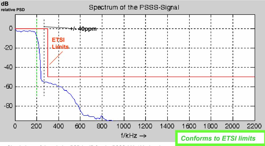
Simulations of the relative PSD in dB for the PSSS 250-400 signal: With precoding, at 400 kchip/s, 250 kbit/s, +/- 40ppm, 50% PA drive, as specified in draft TG4b PHY text
