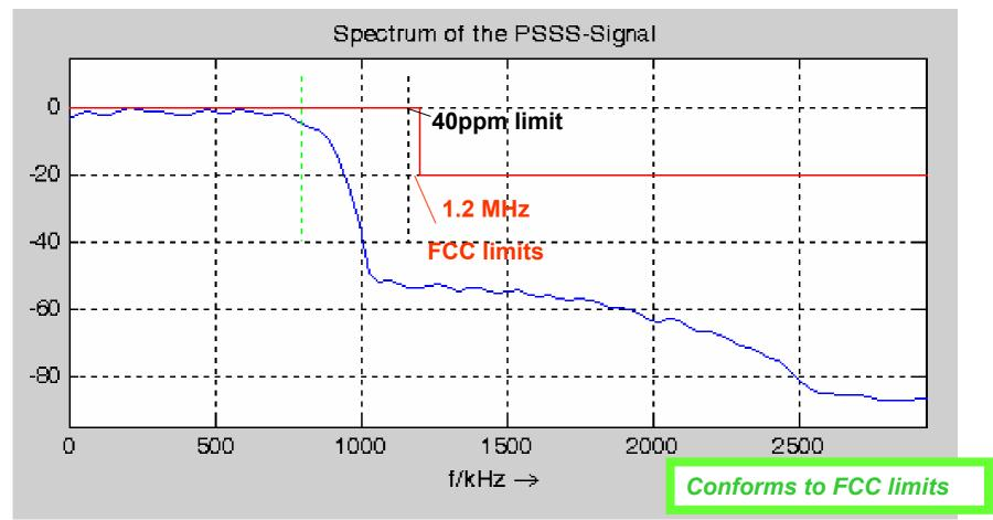
Simulations of the relative PSD in dB for the PSSS 250-1600 signal: With precoding, at 1,600 kchip/s, 250 kbit/s, +/- 40ppm, 50% PA drive, as specified in draft TG4b PHY text
