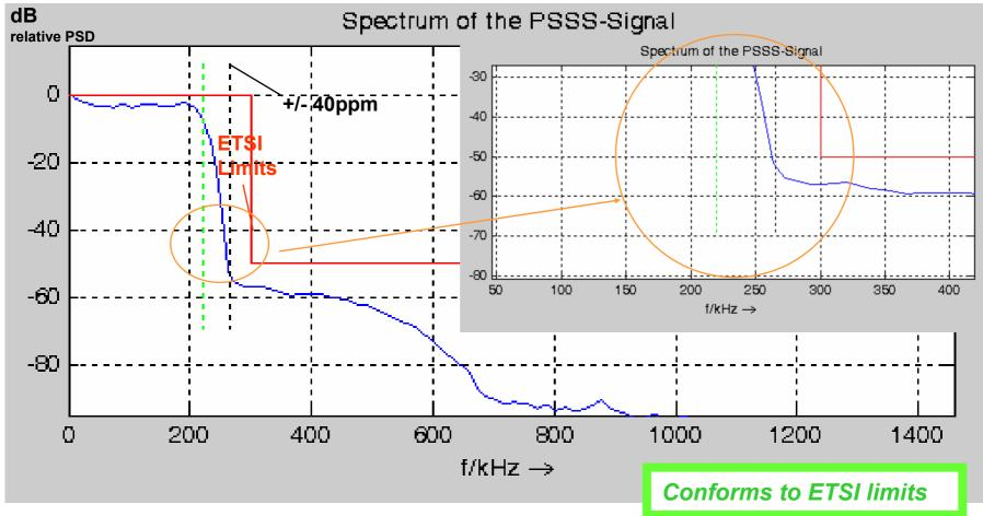
Simulations of the relative PSD in dB for the PSSS 206-440 signal: With precoding, at 440 kchip/s, 206 kbit/s, +/- 40ppm, 50% PA drive, as specified in draft TG4b PHY text
