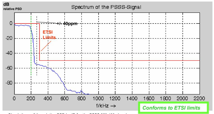
Simulations of the relative PSD in dB for the PSSS 250-400 signal: With precoding, at 400 kchip/s, 250 kbit/s, +/- 40ppm, 50% PA drive, as specified in draft TG4b PHY text
