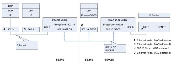
Figure 8: Example LAN with 4 endpoint nodes: A, B, C, D
