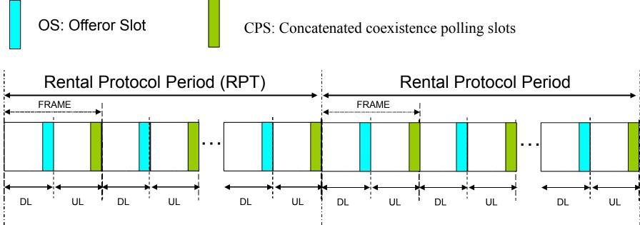
– In each RPT, N OS are available to any O-BS if needed. Different O-BSs can establish RF link with specific R-BS via LLC to enable CTCP. Each O-BS chooses an available OS.
