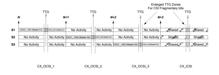
Figure 3: Allocation of CXCC Frames for Control sub-frame Usage
