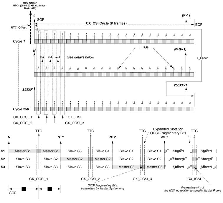
Allocation of Fragmentary Bits for ICSI and OCSI signalling
