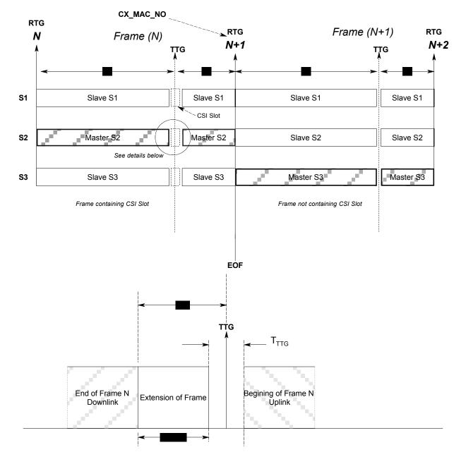
OCSI Fragmentary Bit=1 when Frame extends into DL\_CSI OCSI Fragmentary Bit=0 when Frame does not extend into DL\_CSI
