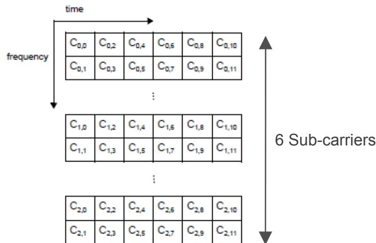
Figure 555—PFBCH comprised of three distributed 2x6 UL FMTs
