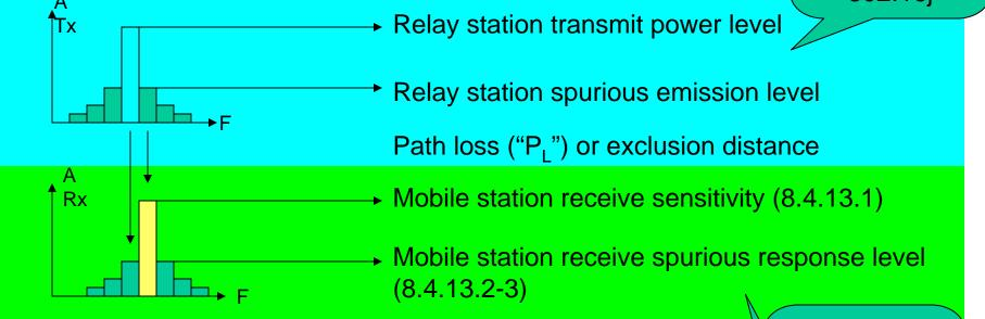
After choosing a suitable exclusion distance and path loss, then the allowed emissions from the relay station can be calculated from the 802.16 receiver performance requirements These parameters are already set in 802.16 2006-05-01
