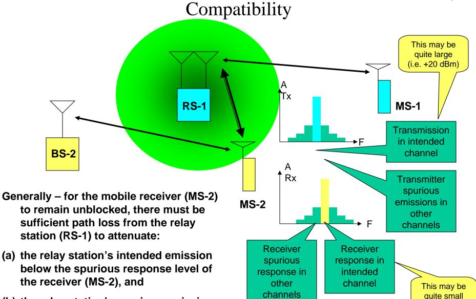
(b) the relay station's spurious emissions below the minimum receiver sensitivity (or received signal level).
