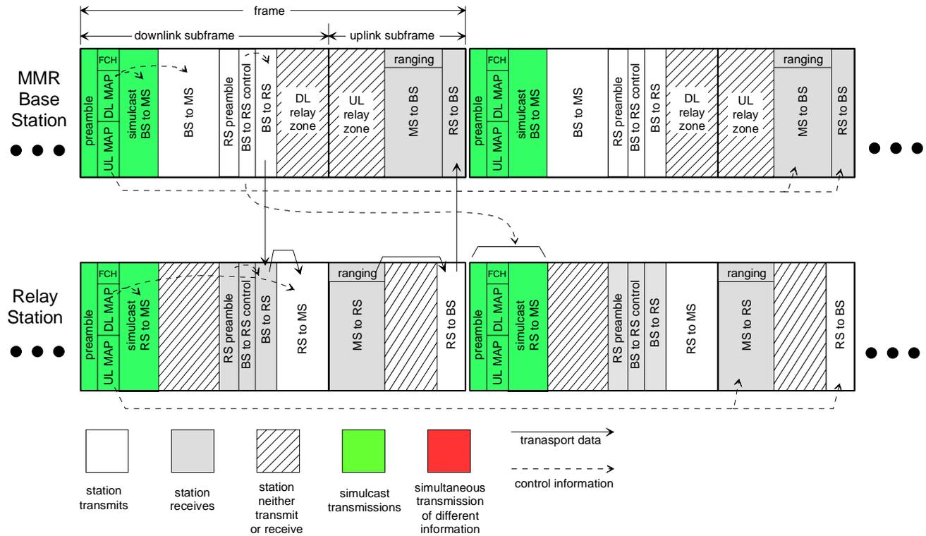
Figure 5. Frame Structure 3 using simulcast transmission
