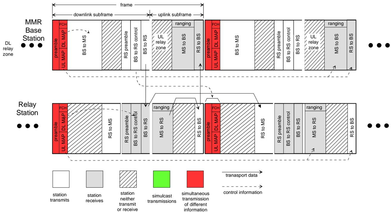
Figure 4. Alternative Frame Structure 2c
