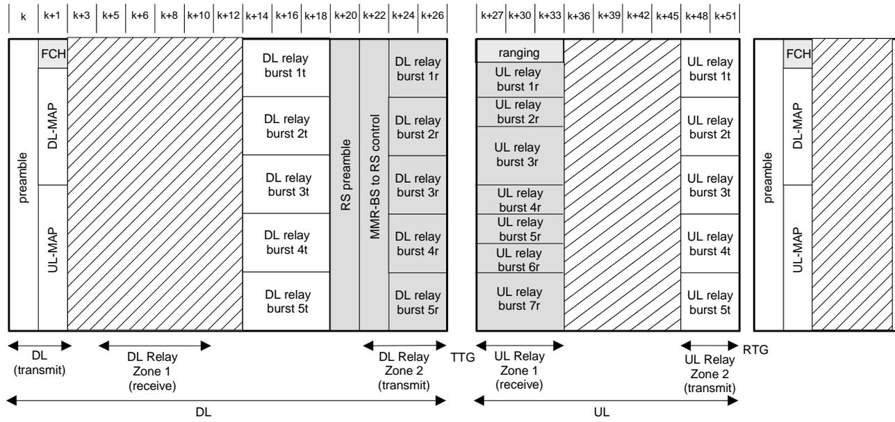
Figure 13. Frame Structure 2c from point of view of the RS (option 3).
