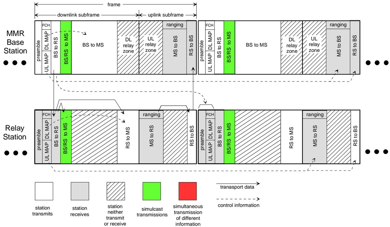
Figure 6. Frame Structure 4 without RS preamble
