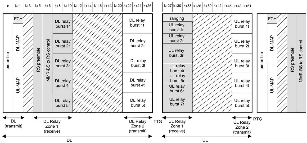
Figure 11. Frame Structure 2b from point of view of the RS (option 2).
