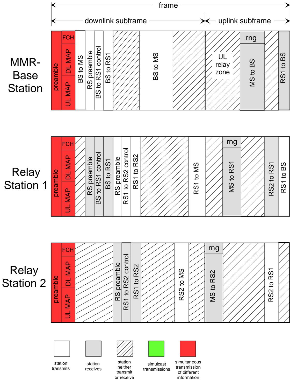
Figure 7. Extension of recommended frame structure to support multiple hops.
