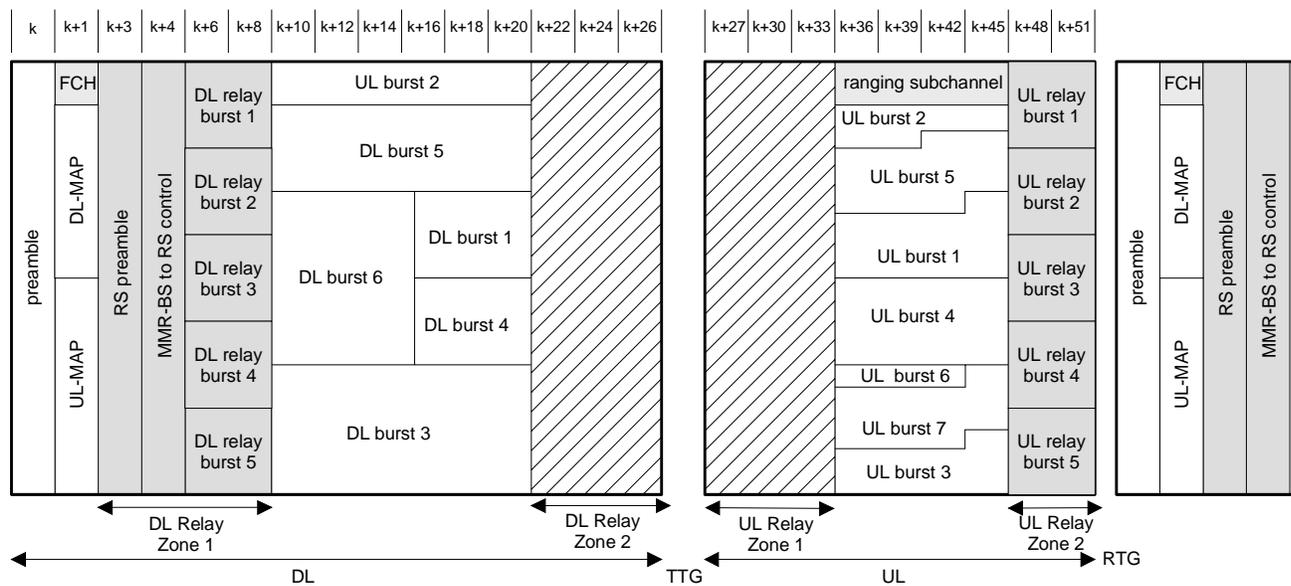
Figure 8. Frame Structure 2a from point of view of the MMR-BS (option 1)
