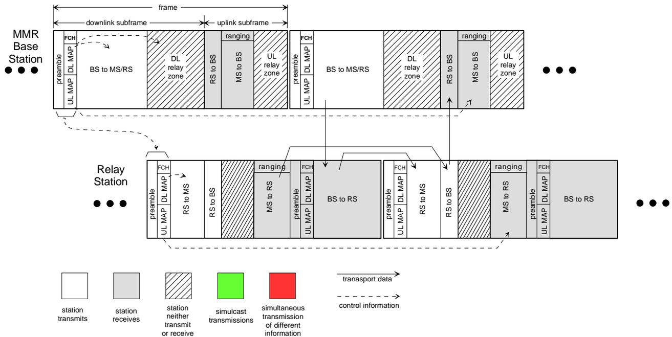
Figure 1. Frame Structure 1 with time offset preambles for RS
