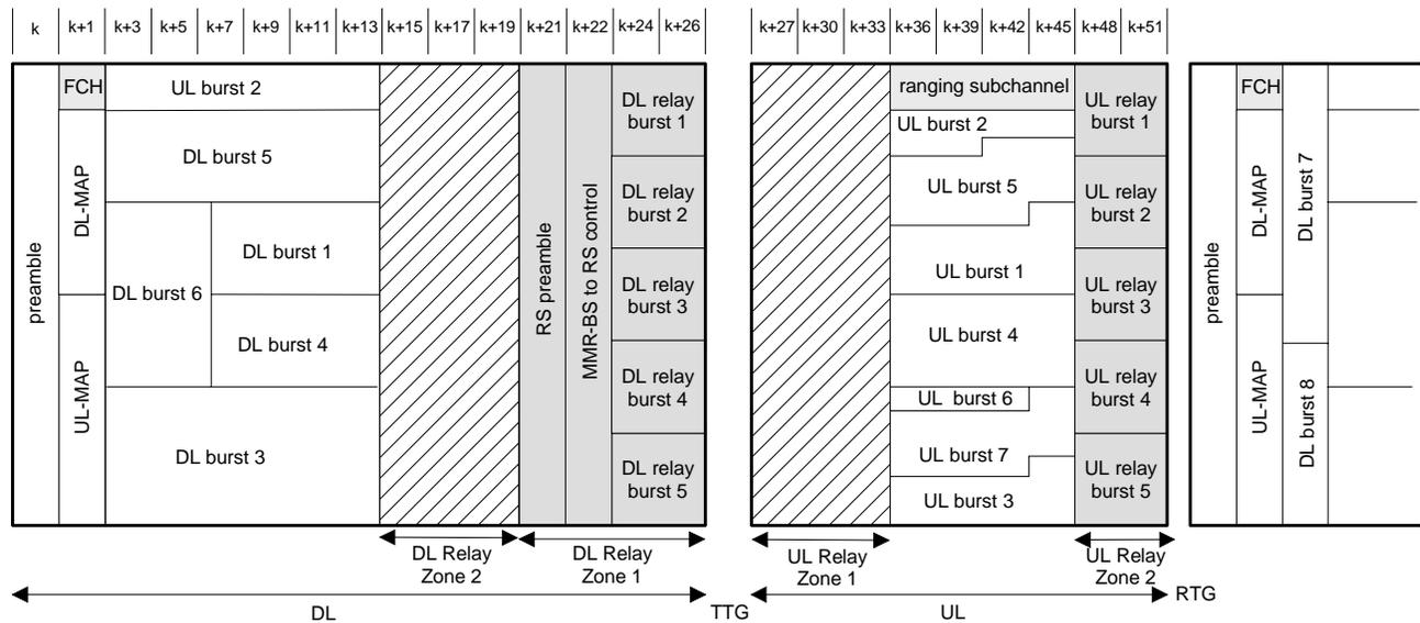
Figure 12. Frame Structure 2c from point of view of the MMR-BS (option 3)
