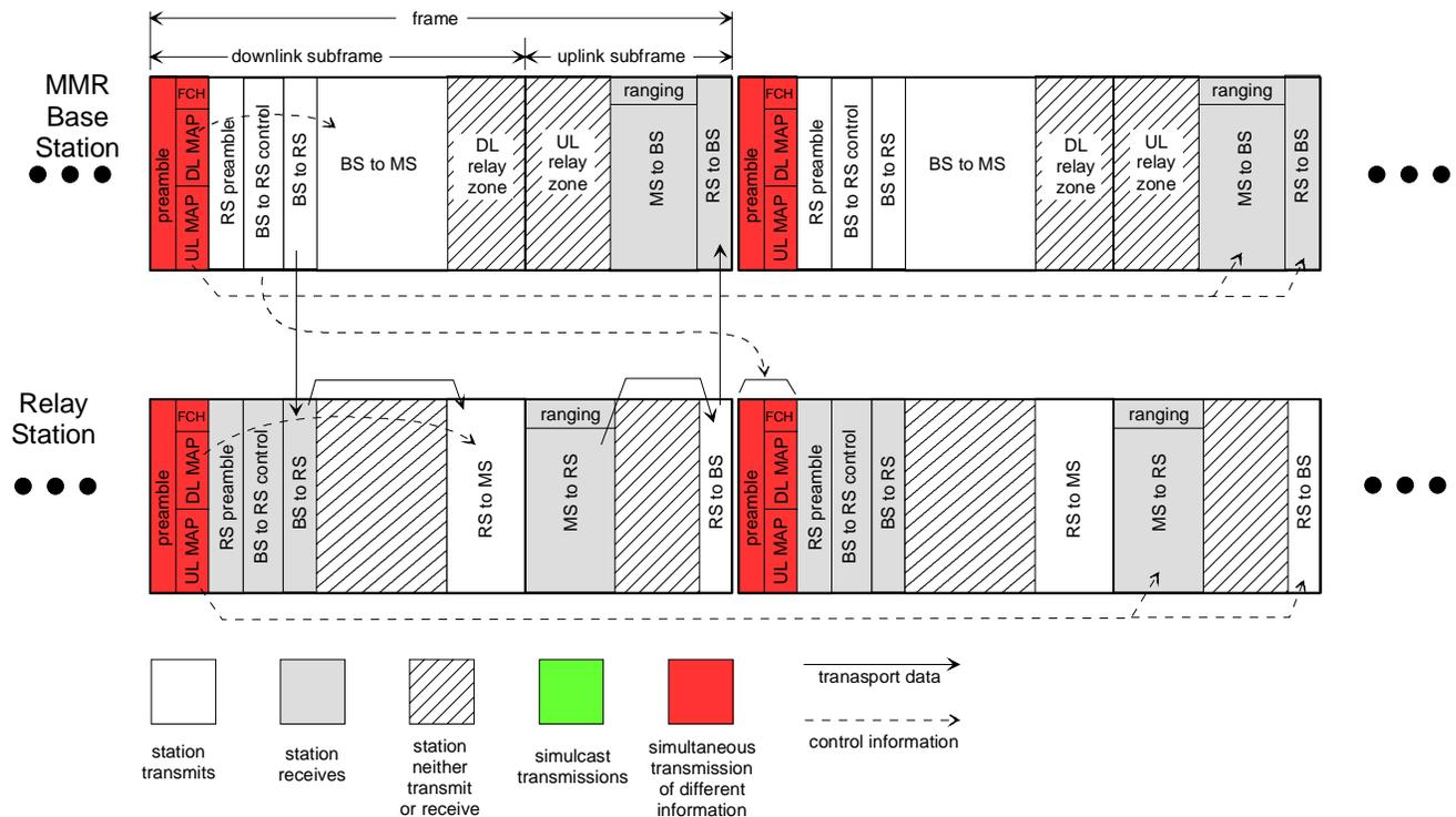
Figure 2. Frame structure 2a with synchronized preambles
