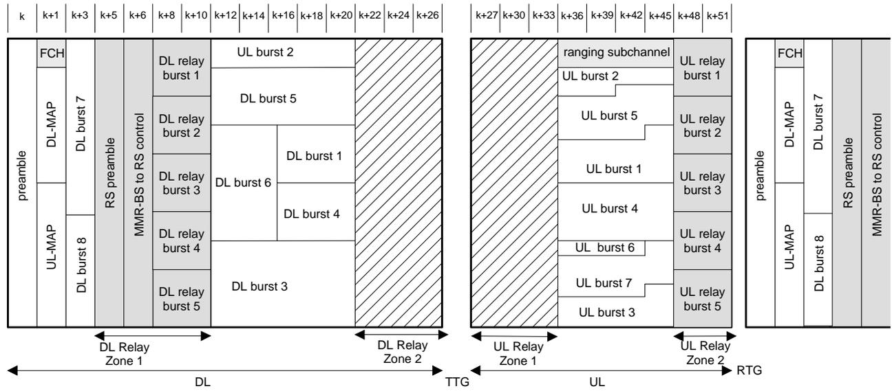
Figure 10. Frame Structure 2b from point of view of the MMR-BS (option 2)
