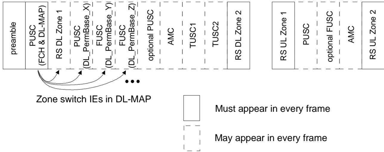
Figure zzz. Illustration of OFDMA relay frame with multiple zones
