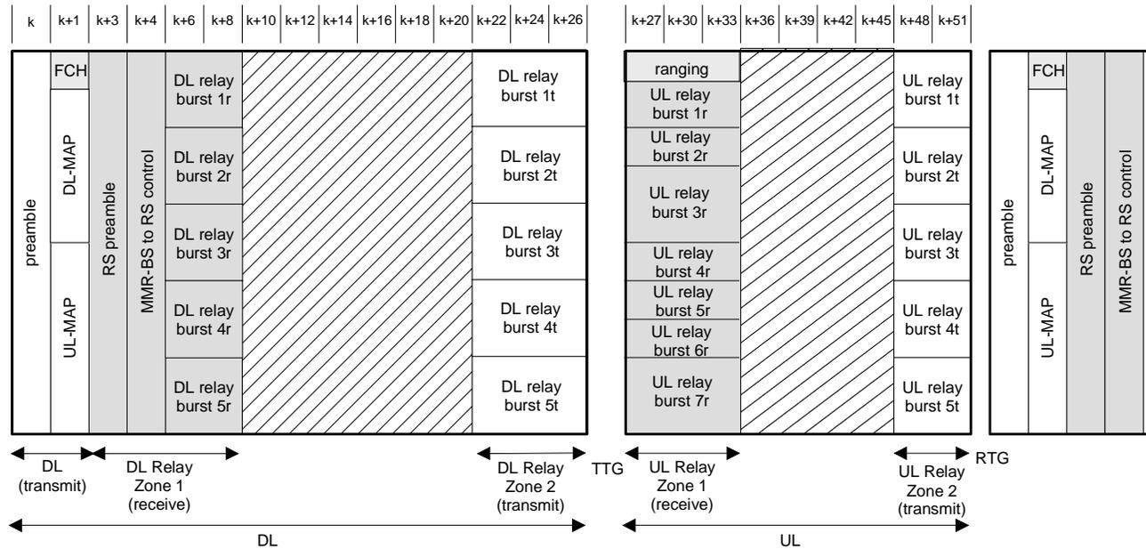
Figure 9. Frame Structure 2a from point of view of the RS. (option 1)
