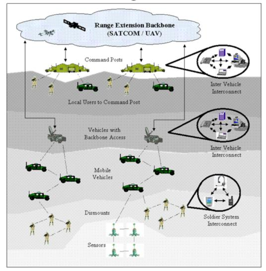
• BS/relay mobility, mobile multi-hop relaying, and security are unique requirements for the military to deploy 802.16e
