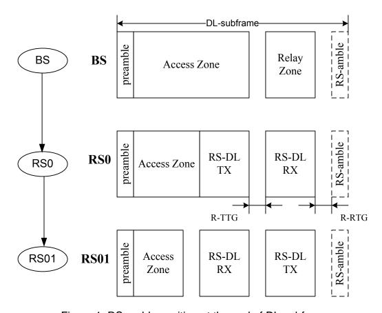
Figure 1. RS-amble position at the end of DL-subframe
