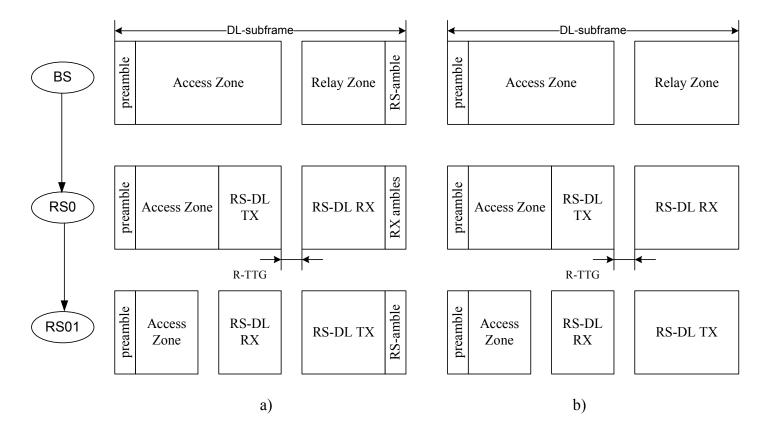
Figure 2. Examples of re-using the RS-amble and transition gaps symbols
