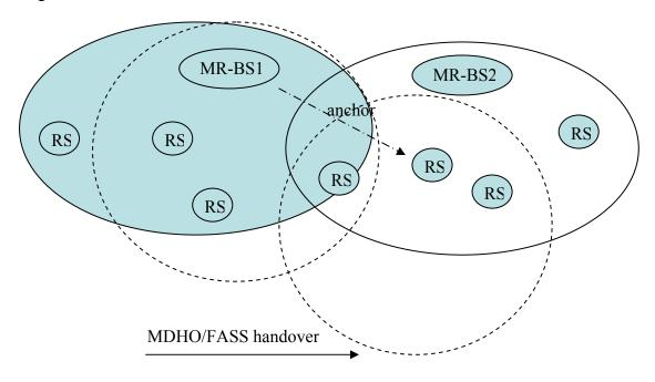
Figure 7: Inter MR-BS handover, the current anchor station is MR-BS and target anchor station is RS controlled by the different MR-BS
