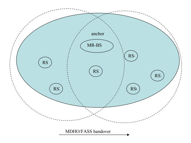
Figure 1 : Intra MR-BS handover, the current anchor station and target anchor station is the same MR-BS  $\,$
