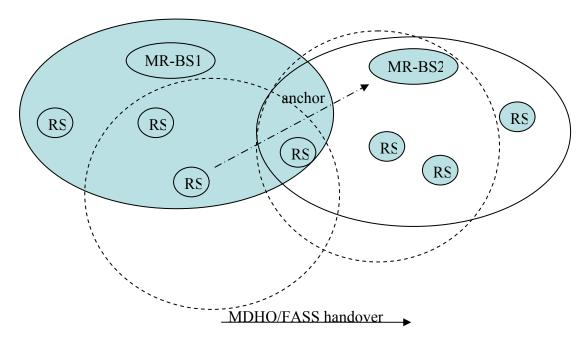
Figure 8 : Inter MR-BS handover, the current anchor station is RS and target anchor station is MR-BS in a different MR-cell
