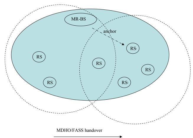
Figure 3: Intra MR-BS handover, the current anchor station is MR-BS and target anchor station is its RS 4 in the same MR cell
