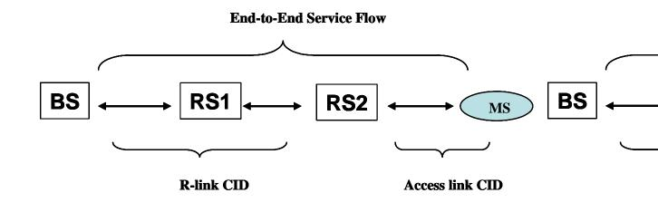
Figure 1 Relay interface over R-link and the access interface over access link
